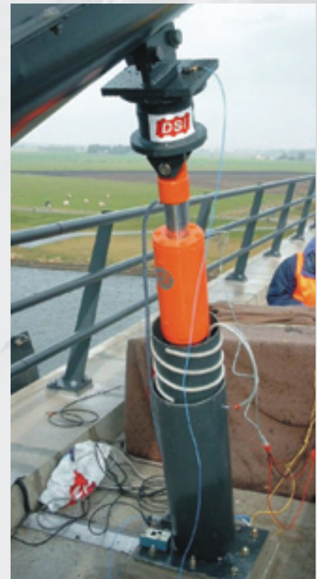
Test Installation of a Hydraulic Damper
